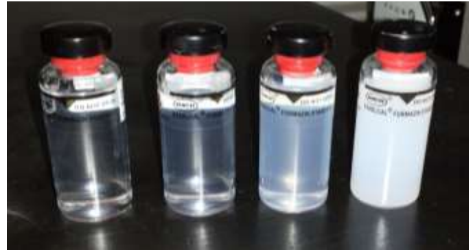
Figure 1: Examples of solutions with varying turbidity, from left to right: 10 NTU, 20 NTU, 100 NTU, and 800 NTU (photo credit: HMGA)
