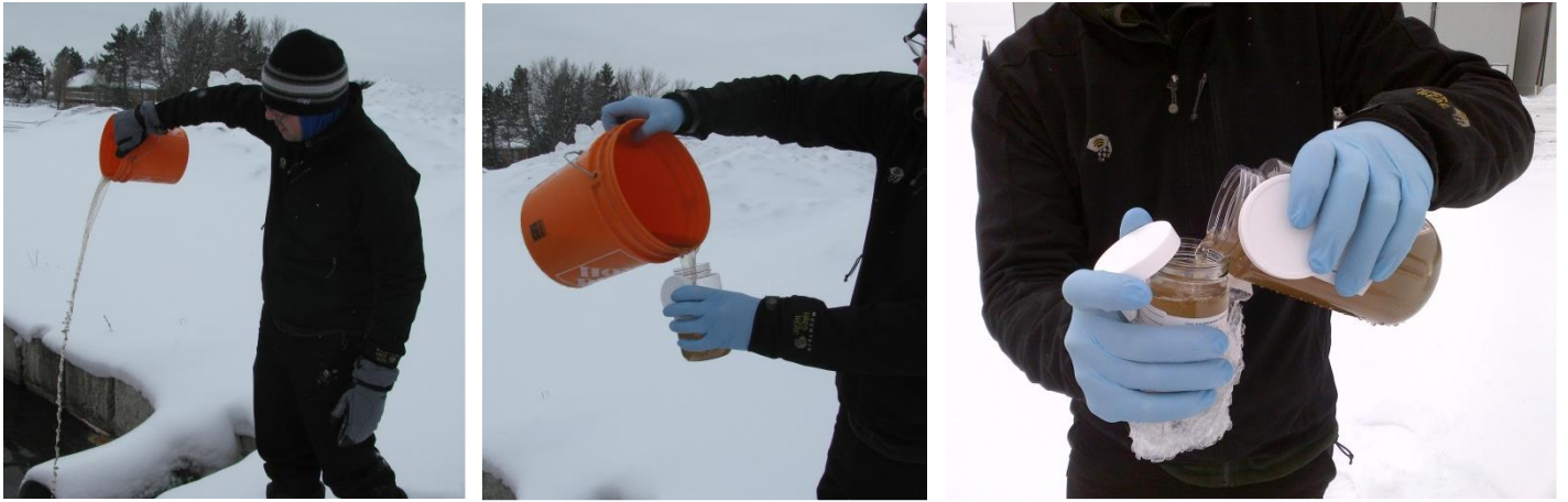
Figure 2: Sampling Procedures include rinsing the bucket (left), decanting into a sample bottle (centre), and decanting into a secondary sample bottle (right)
