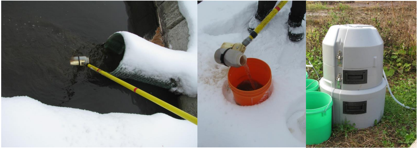
Figure 1: Sampling equipment include a telescopic sampling pole collecting water (left), combining samples into a bucket (centre), and an Auto-sampler (right)
