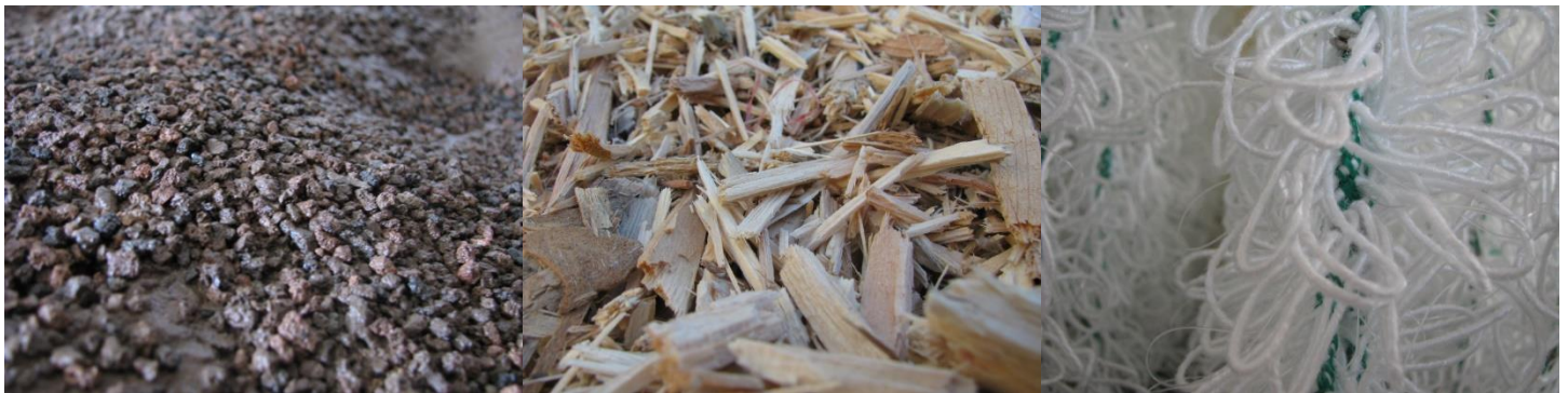
Figure 1: Examples of media in a biofilter; lava rock, an inert material (left), woodchips, an organic material (center), and synthetic cording, a man-made material (right)
