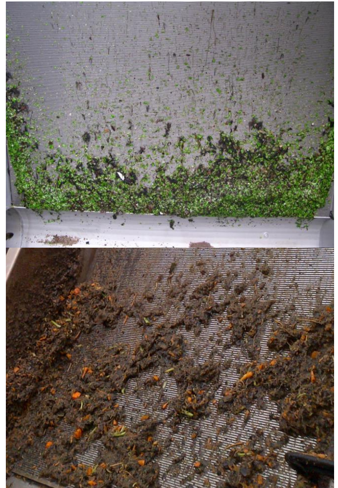
Figure 4: Solids collected by parabolic filter screen (top) and a hydro-sieve (bottom) (Photos: HMGA Water Project)
