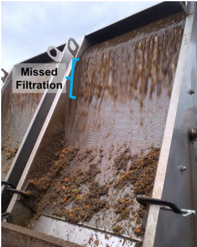
Figure 3: An example of a hydro-sieve that is not running at full capacity (Photo: HMGA Water Project)
