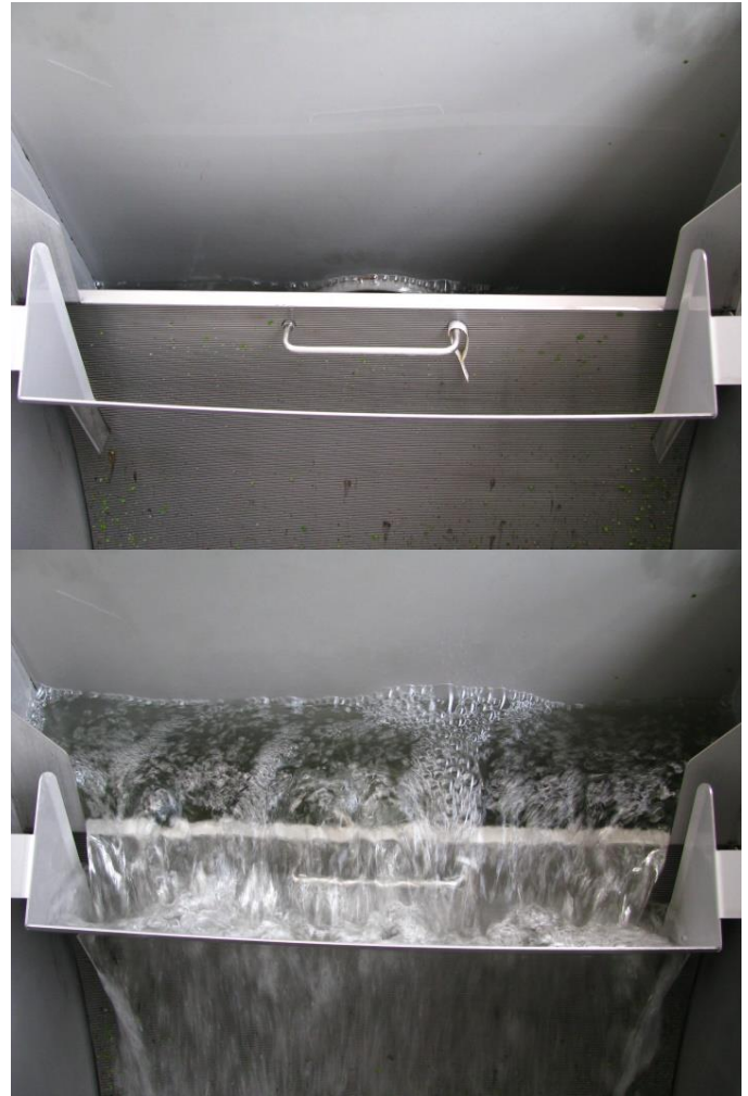
Figure 2: A parabolic filter screen fitted with a plate to direct the water flow onto the screen; no water flow is shown on the top and water flowing through on the bottom (Photo: HMGA Water Project)
