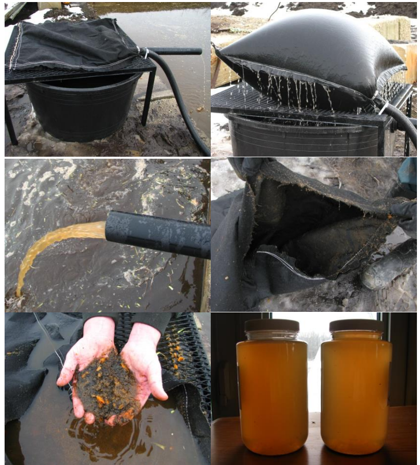
Figure 1: Filter bag test rig (top left), test in progress (top right), outflow from filter bag into settling pond (middle left), bag ruptured at seam (middle right), solids filtered by bag (bottom left), and water samples from inflow on left and outflow on right (bottom right)
