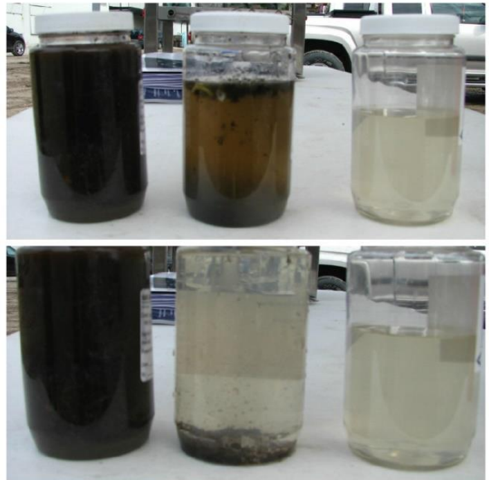
Figure 4: Water samples prior to treatment (left), immediately following the addition of coagulants and flocculants (middle), and post-Geotube® (right). The top and bottom pictures were taken approximately 1 minute apart, demonstrating the speed of settling once the solids have flocculated.
