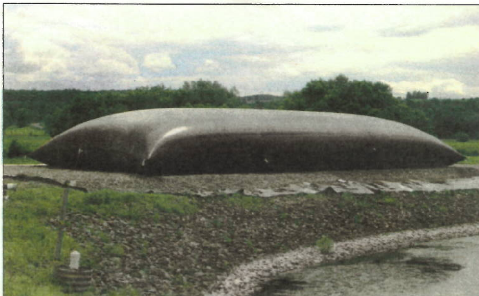
Geotube dewatering system
