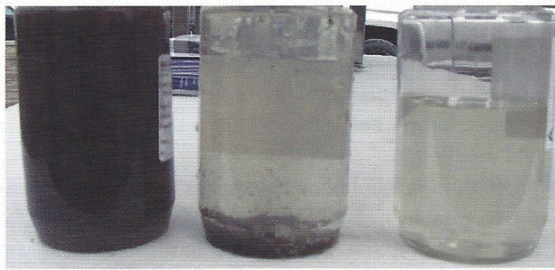
PRE-TREATMENT (LEFT), WATER TREATED WITH COAGULANTS AND FLOCCULANTS (MIDDLE) AND POST-GEOTUBE® (RIGHT) WITH TOP AND BOTTOM PICTURES TAKEN APPROXIMATELY 1 MINUTE WITH THE ADDITION AND MIXING OF COAGULANTS AND FLOCCULANTS.
